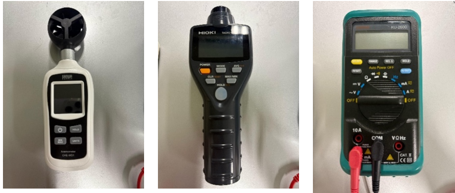
(a) (b) (c) Fig. 3.10 Anemometer (a), Tachometer (b), and Multimeter (c)
