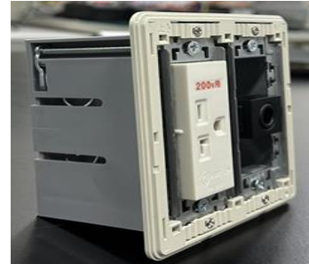
Figure 5. Panel box in which the PCB is to be fitted
