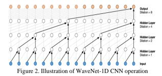
The input feature for the WaveNet model is the optimal time-lagged energy consumption data. The filters in the input layer compute the weighted sums and biases and pass their output as an input to the dilated hidden layer and the process is repeated. Table I is a summary of the hyperparameters used to design the WaveNet model.
