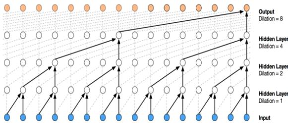
Figure 2. Illustration of WaveNet-1D CNN operation
