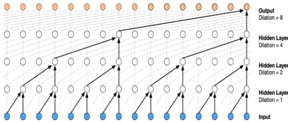
Figure 2. Illustration of WaveNet-1D CNN operation
