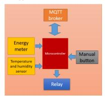
Figure 2 Configuration of the smart metering application
