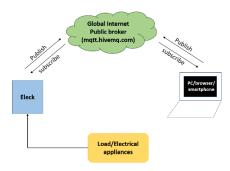
Figure 1 Data process of a smart meter
