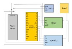
Figure 3 Experimental circuit of smart meter
