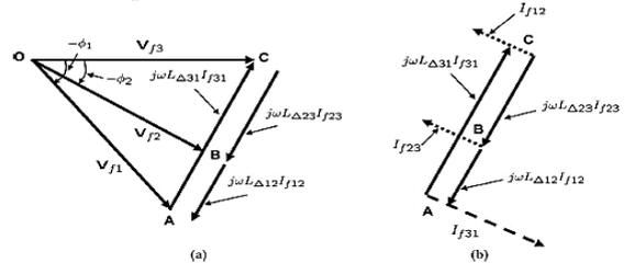
Figure 3. Phasor diagram for HB3 isolation
