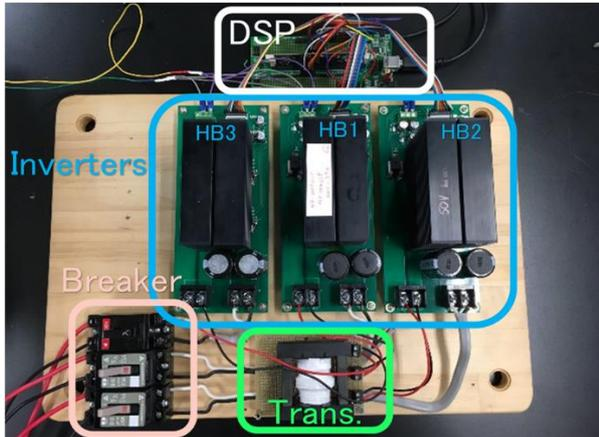
Figure 6. Experimental equipment of TAB converter
