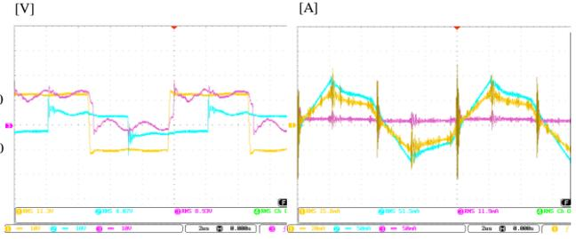
Figure 7. Waveform (Left:  $[v_p, v_{s2}, v_{s1}]$ , Right:  $[i_p, i_{s2}, i_{s1}]$ )
