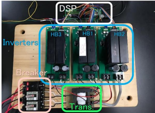
Figure 6. Experimental equipment of TAB converter
