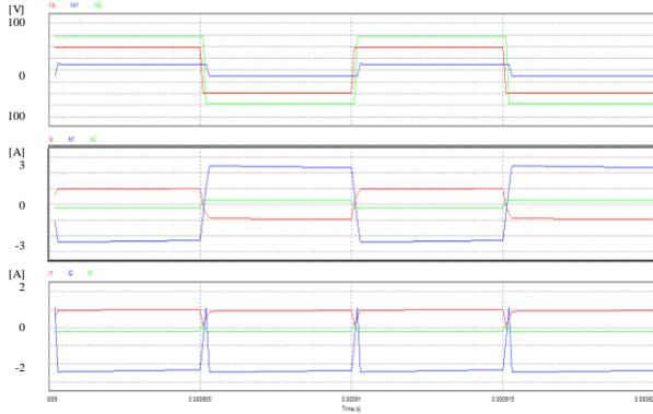
Figure 5. Waveform ( $[v_p, v_{s1}, v_{s2}]$ ,  $[i_p, i_{s1}, i_{s2}]$ ,  $[I_1, I_2, I_3]$ )
