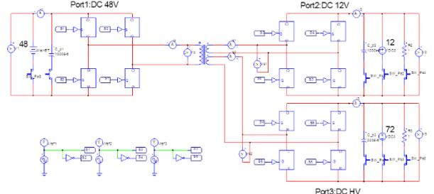
Figure 4. Simulation circuit
