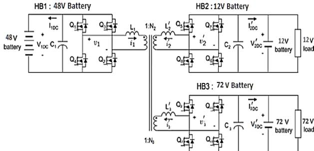
Figure 1. Model circuit of TAB converter
