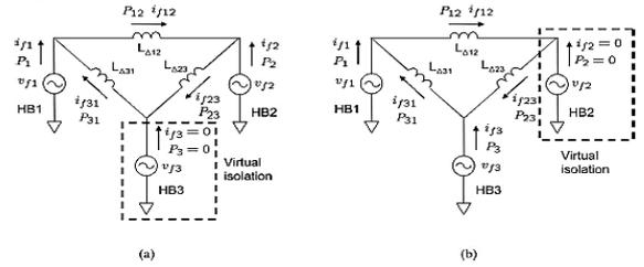
Figure 2.  $\Delta$ -equivalent circuit for HB3 and HB2 isolation
